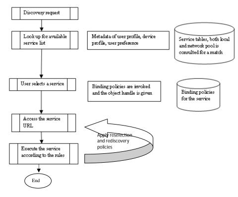
Fig. 5: Service Discovery and Provisioning
